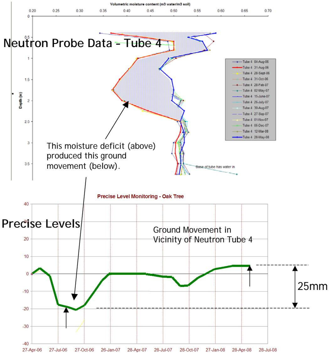
The green line (bottom) plots the ground movement in the vicinity of the neutron probe over time. The difference between August 2006 and May 2008 amounts to around 25mm. The blue shaded area of the top graph (representing the loss of moisture between the two readings) has produced 25mm of ground movement.
