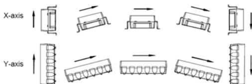
The sensor measures tilt in two directions (see above) and has a claimed resolution of 0.001 degrees. Hopefully the new and cheaper technology will raise industry interest.
